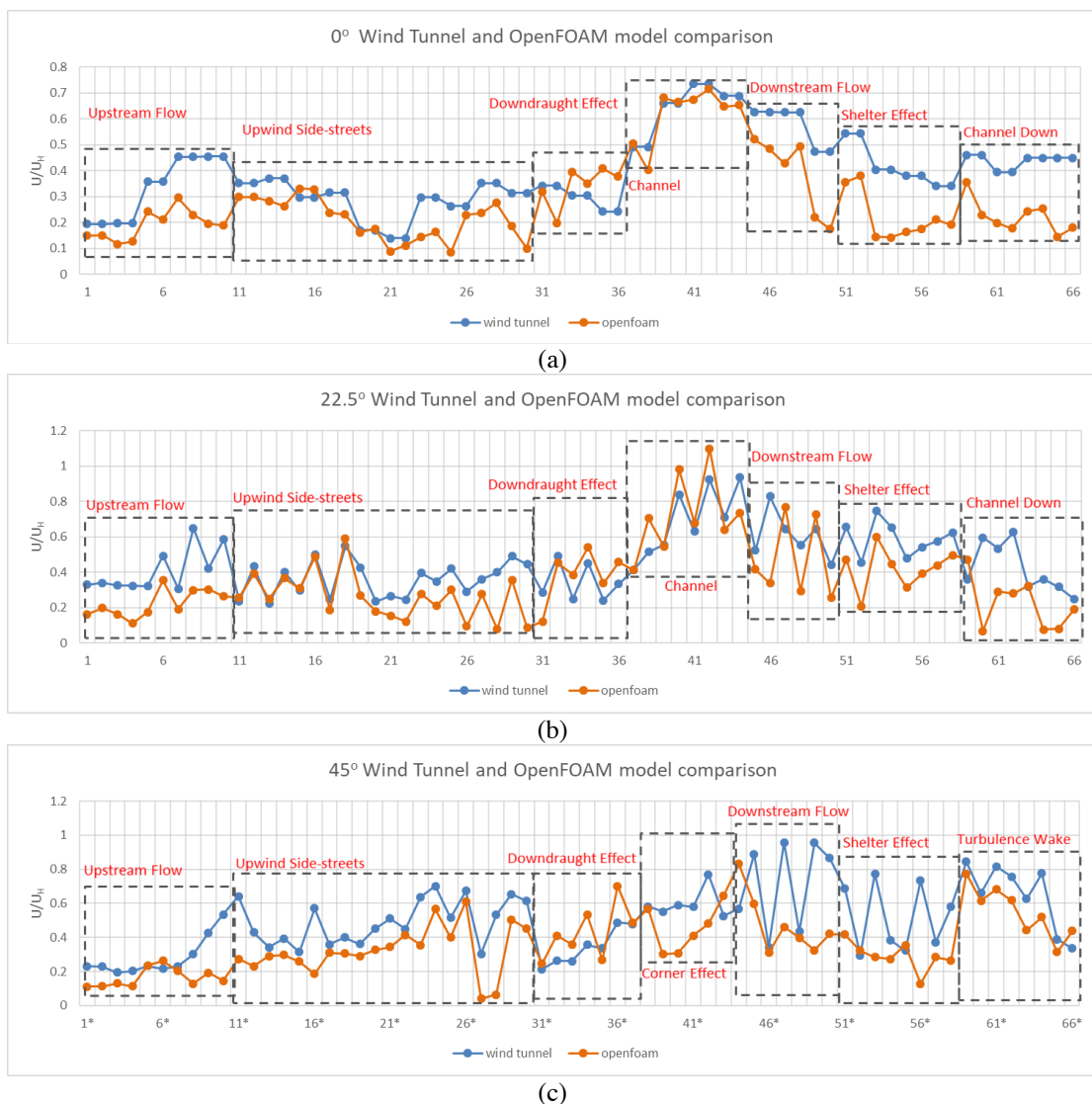
Figure 25: Comparison of wind speed ratios at different wind direction
