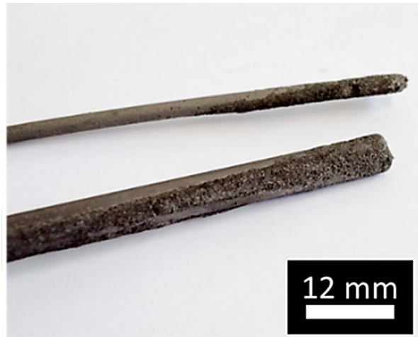
Figure D.11 the photograph of the sampling tube showing a small quantity adhered particles to the tube.
