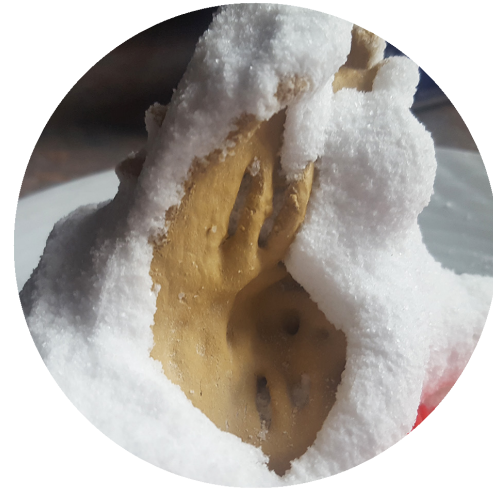
Figure 2.14: 3D print coated in slip and baked
