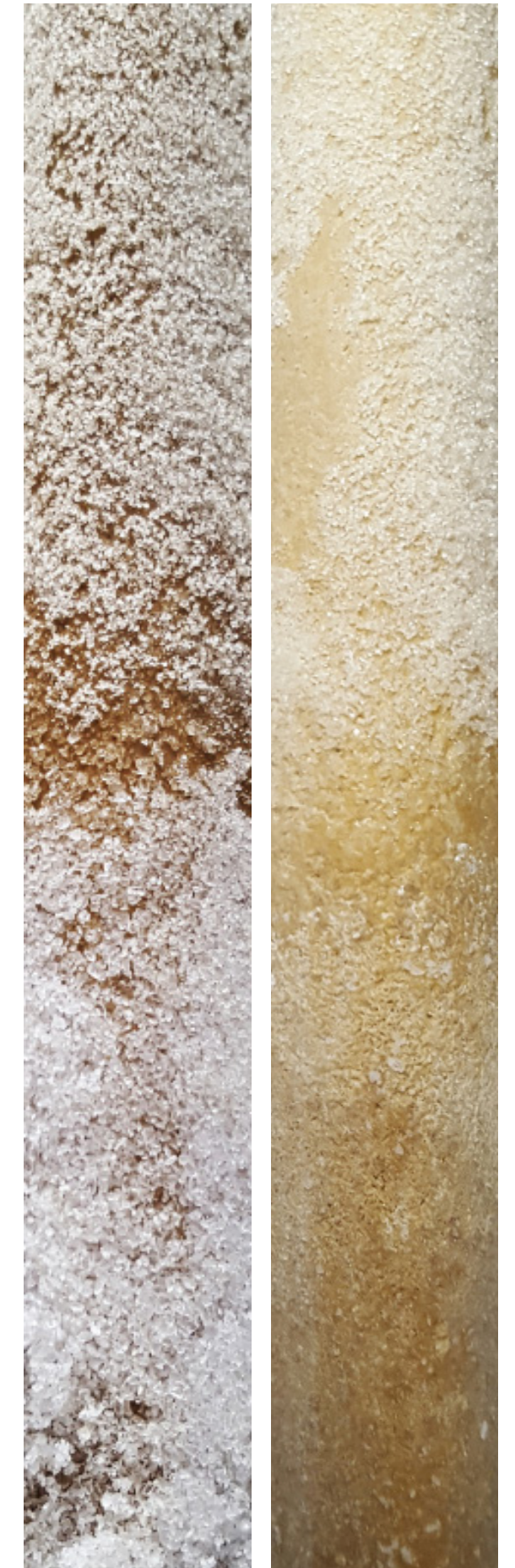
Figure 2.05: Gradient in curing example
