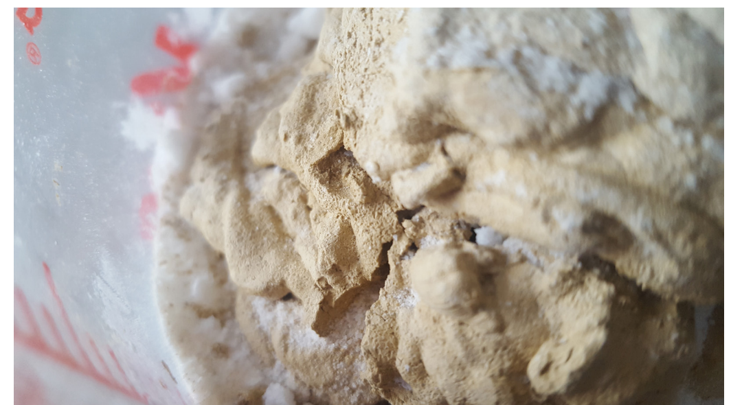
Figure 2.15: Cracking in 'printed' clay body as a result of encasement
