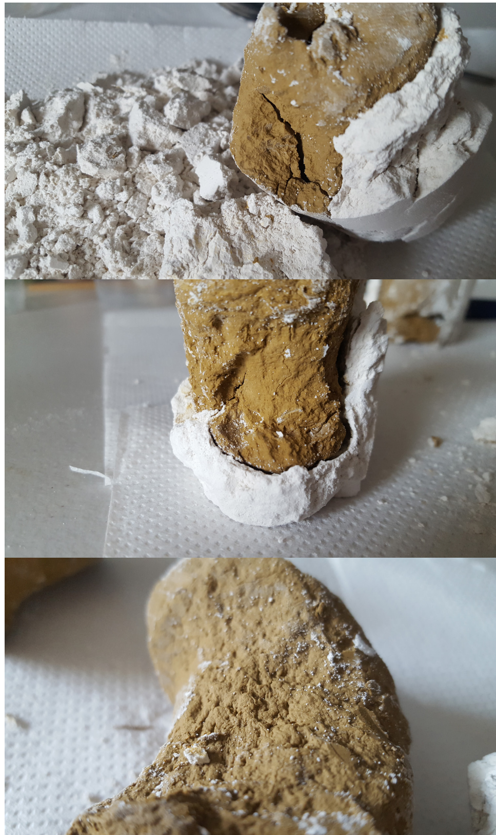
Figure 3.02: High pressure extrusion into plaster
