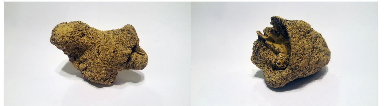
Figure 3.03: High pressure extrusion into sand
