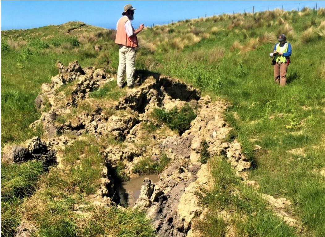
Figure 3.7: Fissured, bulged up moletrack at the paleoseismic trench site along the Napoleon segment, shown in Figure 3.2a. Russ Van Dissen is pictured (centre) standing on the largest intact turf raft at the site (see also Figure 3.14); the rest of the up-bulged material is fairly jumbled and disorganised. This is partially because the sub-surface material is backfill from the original trench excavation, which more easily detached from its roots (see Chapter 4 of this thesis for further detail). Photograph taken by Mark Hemphill-Haley, 23/11/2016.
