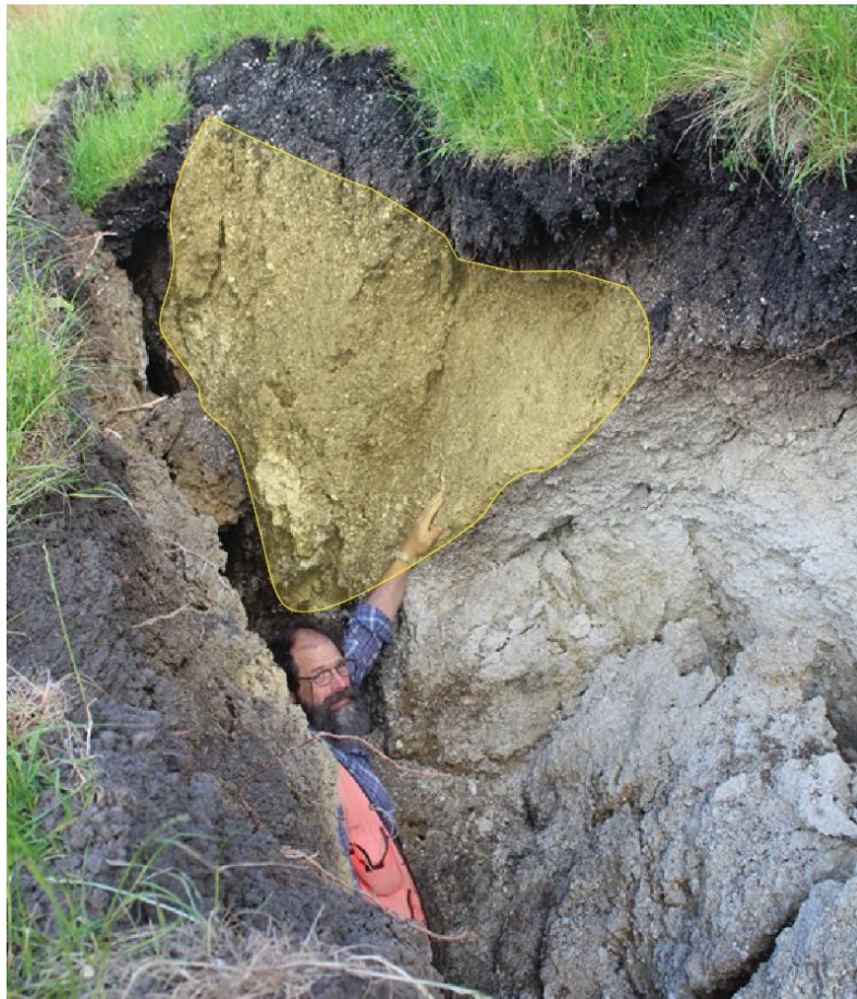
Figure 2.5: Paleofissure that re-opened during the 2016 earthquake, located ~100 m southwest of Trench 1 along fault strike, and ~25 m southwest of Trench 3 along fault strike (see Figure 2.2). Infill of the paleofissure is shaded yellow, whereas the deepened cavity that opened in 2016 is what the geologist is occupying. Three radiocarbon samples were taken from the shaded area of this fissure, which were used to constrain an older paleoearthquake, E5 (see section 2.3.2.4). Photograph taken by Kate Clark, 27 th of November 2016.
