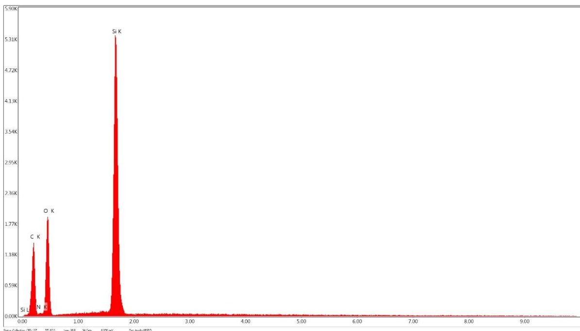
Figure 8.49. EDS spectrum (counts vs keV) of Batch 4 CnGmSiO 2 /epx (free ligand) coating (200× magnification, HV 20 kV, spot size 6, WD 10 mm, 30 s live time, 1.6 μs amplitude time, 35.1° take-off angle, 129 eV resolution).
