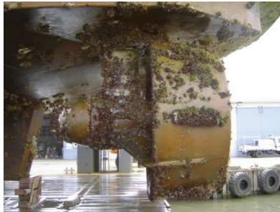
Figure 1.2. Biofouling on ship hulls. 23
