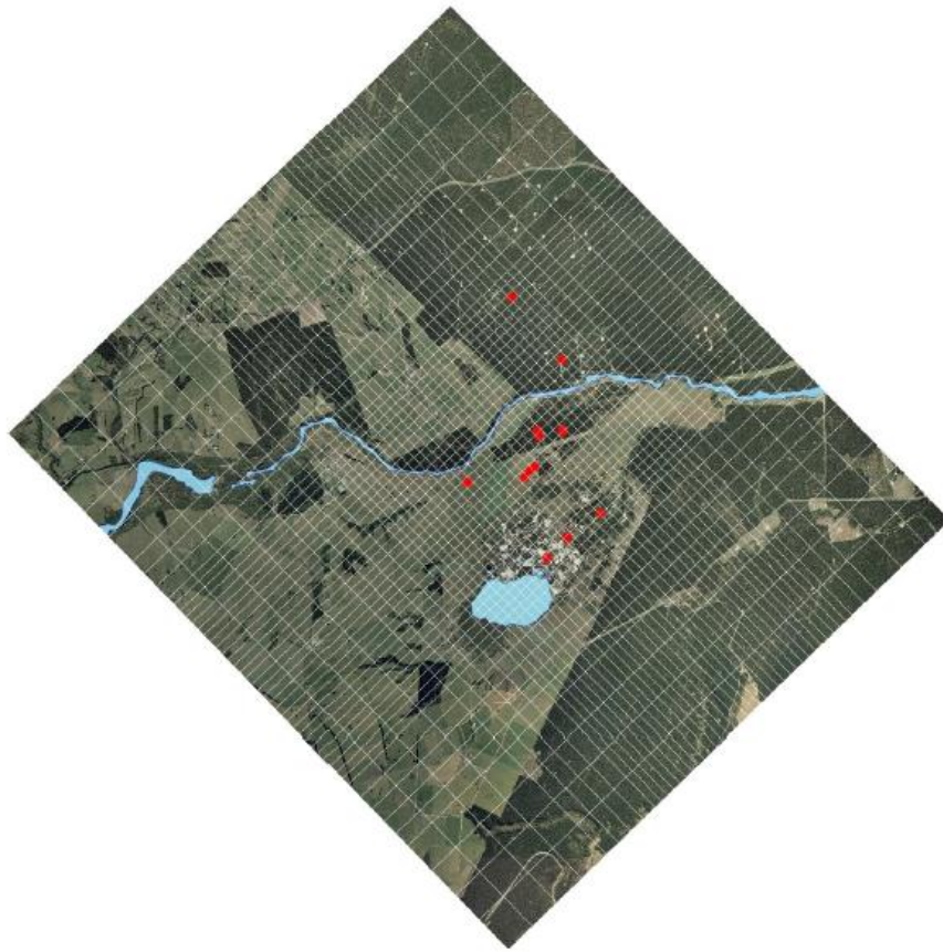
Figure 18: Aerial photo of the Rotokawa region that is included in the numerical model. The yellow lines are the borders of computational grid blocks.
