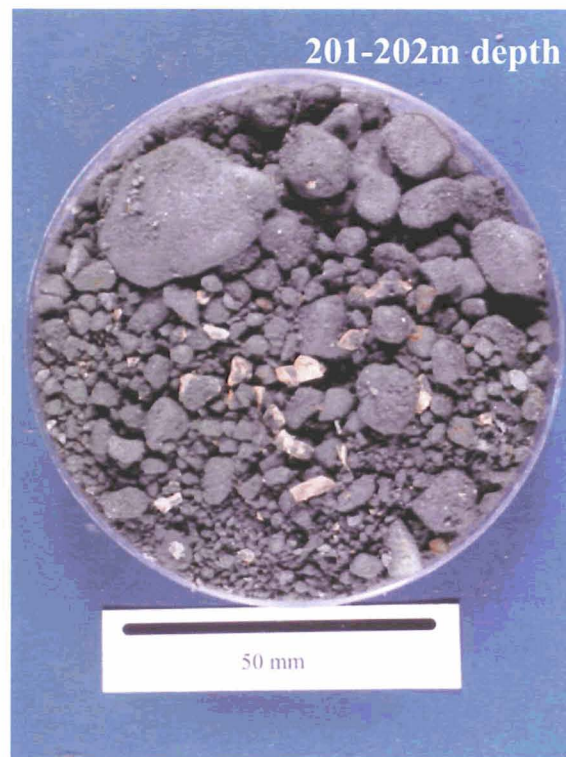
Figure 3.6: Photographs of lithologies consisting of Facies SL (top) and SG (bottom). Facies SL (Sample 223-224m depth) is shell rich and formed on a terrigenous starved inner shelf environment (i.e. Mid cycle shell bed of Abbott, 1997). Facies SG (sample 201-202m depth) is a shelly gravel which formed in a high-energy innermost shoreface environment possibly upon a wave-cut platform.
