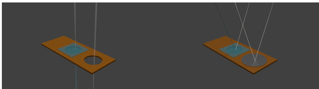
Figure 5.3: Measurements were conducted by mounting the sample on a copper stage inside a LHe flow through cryostat. Transmission measurements (left) were conducted by first measuring the background spectra through a hole in the stage and comparing this to the measurement of the sample. Reflectivity measurements (right) were conducted similarly but with an Al film in the place of the hole to serve as a background.
