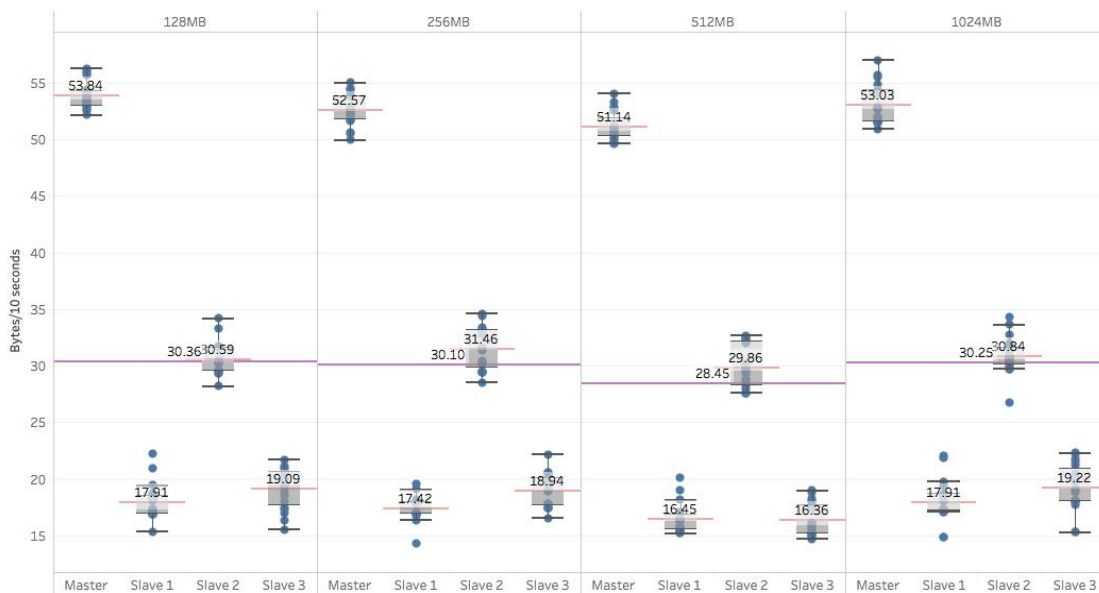
Figure A.4: Box plot and average virtual memory data for 30 runs for different block sizes
