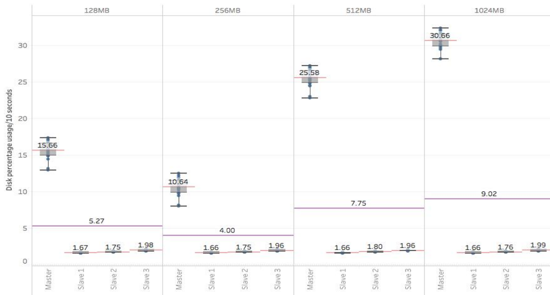
Figure A.3: Box plot and average disk usage data for 30 runs for different block sizes
