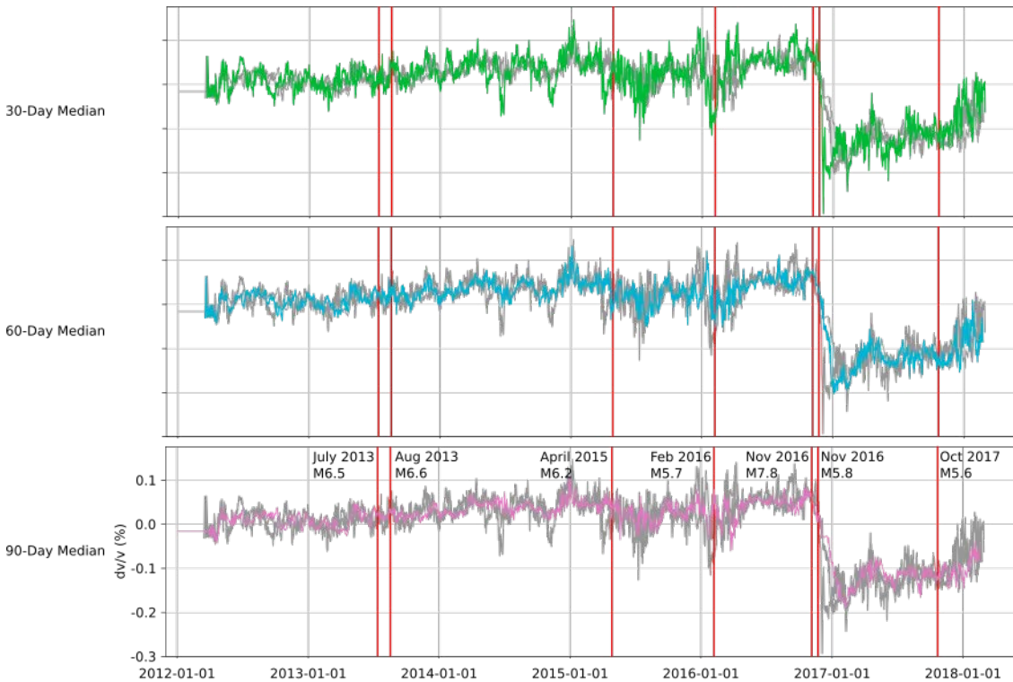
Figure 6.8: Velocity variation plot of median velocity changes for 30-day, 60-day and 90-day moving windows. These windows are the result of the velocity on a given day as the average of the previous N -days including itself. A seven-year reference period was used for the seven-year dataset. The red lines indicate earthquake events with magnitudes greater than 5.6. More details on each earthquake can be found in Table 6.1. Axes values for the top two plots are the same as the bottom plot.
