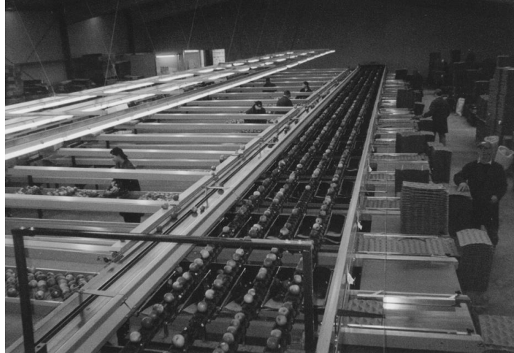
Figure (3.3): A four lane fruit sorting machine
