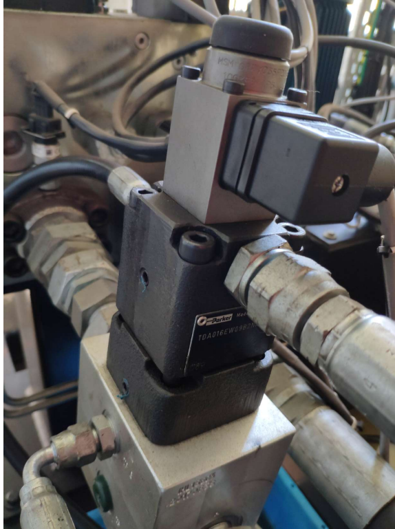
Figure 4.11: TDA016 Proportional throttle valve employed in the ss-CAES prototype.
