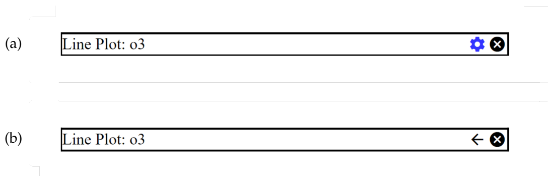
Figure 5.1: The window frame border for the visualizations and the options panel. The top image is the frame for the visualization with a highlighted gear icon which the mouse has hovered over. The bottom image is the frame for the options panel with a back button instead of a gear icon.
