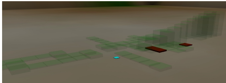
Figure 6.5: Occupied and free space block after robot standing still (at blue mark)
