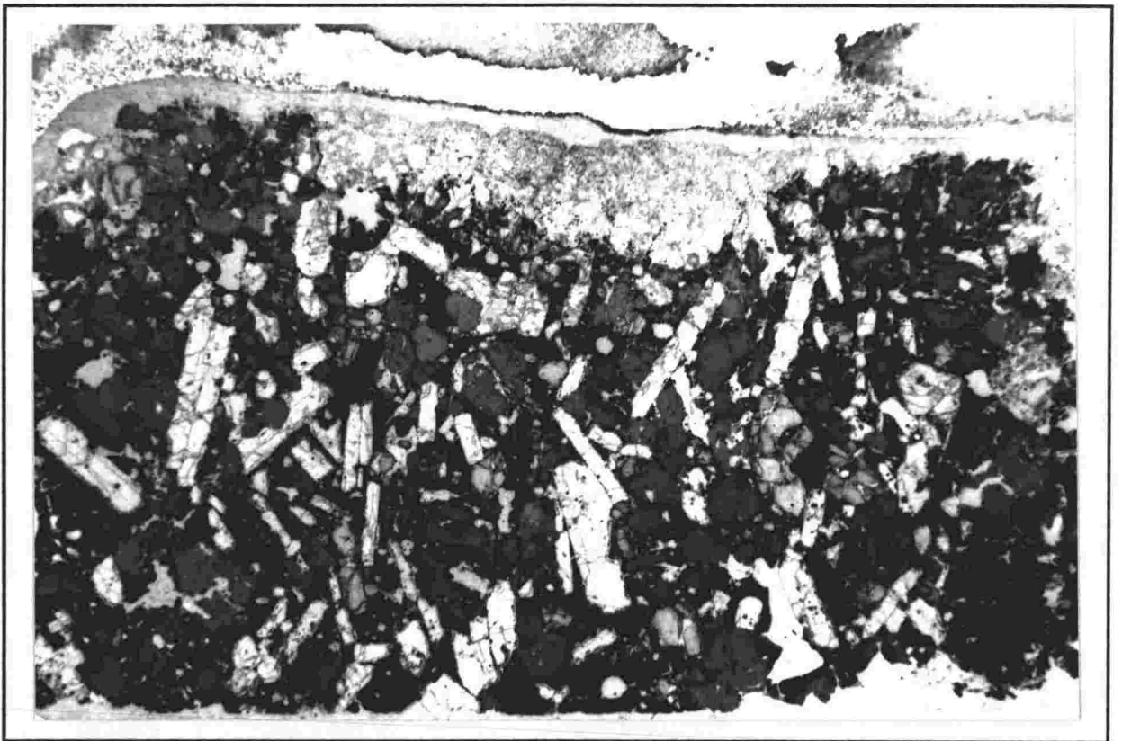
PLATE 6.2: Gabbroic granulite from site 90048 (sample 90048C), consisting of large crystals (many > 2 mm) of euhedral plagioclase (p), olivine (ol), clinopyroxene (c) and Fe-Ti oxides (ox). A rim of host melt (b; bottom right) can be seen to extend only 1-2 mm into the xenolith. Width of plate is 17 mm.
