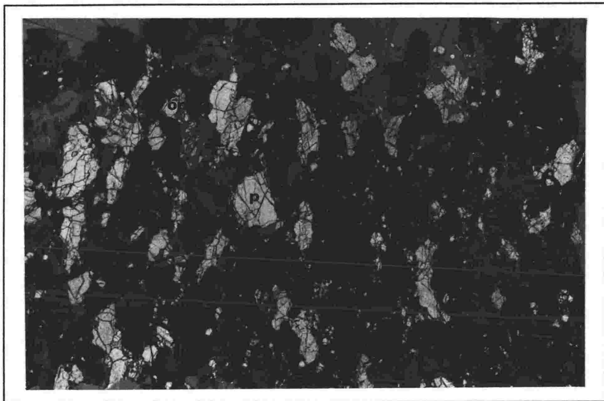
PLATE 4.4: Type M granulite (sample 90029Q) with a layering of mafic phases (clinopyroxene (c) and olivine) and plagioclase (p). Olivine has been wholly oxidised and is opaque (op). Width of plate is 19 mm.
