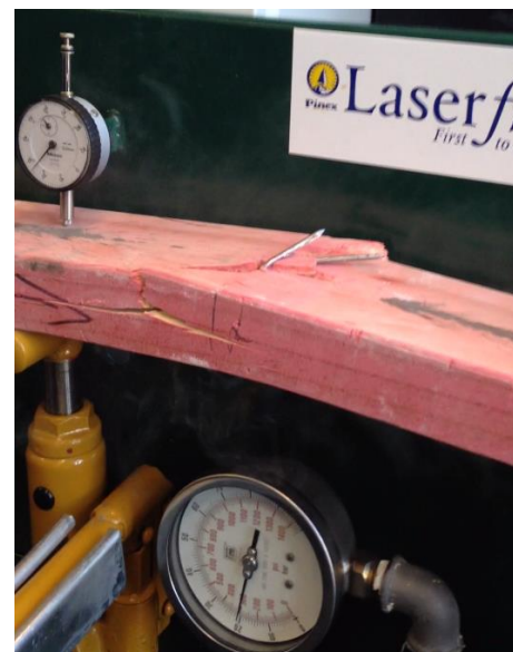
Figure 7 Tested member after breaking point
