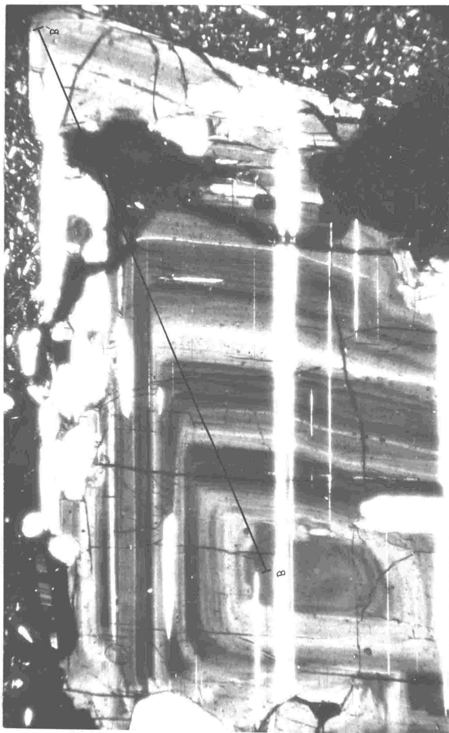
Plate 19. - Photomicrograph of plagioclase phenocryst from sample 11328. A compositional cross-section (B-B') for this crystal is given in Fig. 15. x 65.
