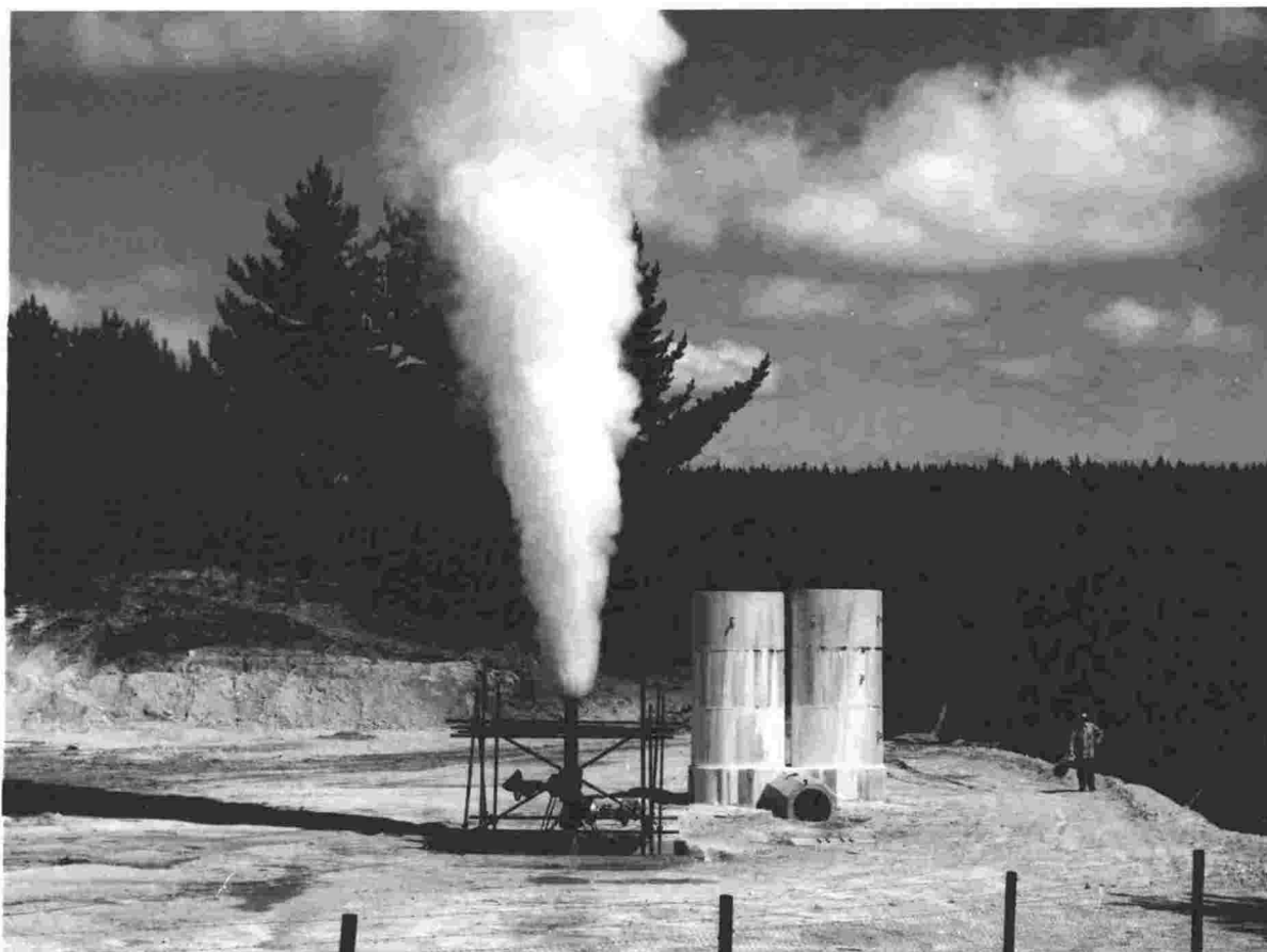
FIG. 7. Bore Br 4 discharging vertically. The mass output of the bore is 51,500 kg/hour at 10 bars pressure. Photo : T.R. Ulyatt.
