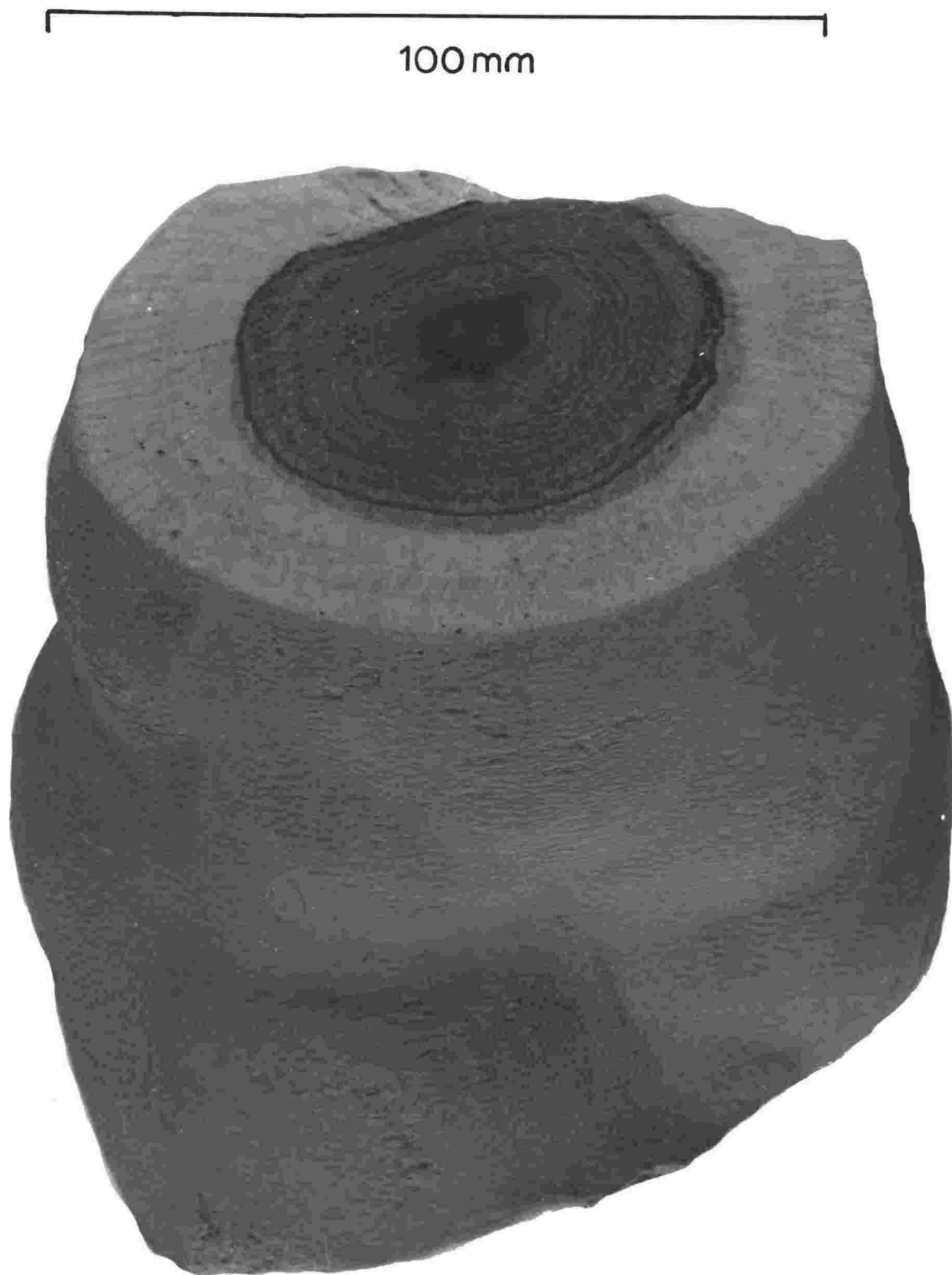
FIG. 10. Aragonite deposited on blackberry stem by water discharged from Br 6. Deposition layers are visible on the cut surface.
