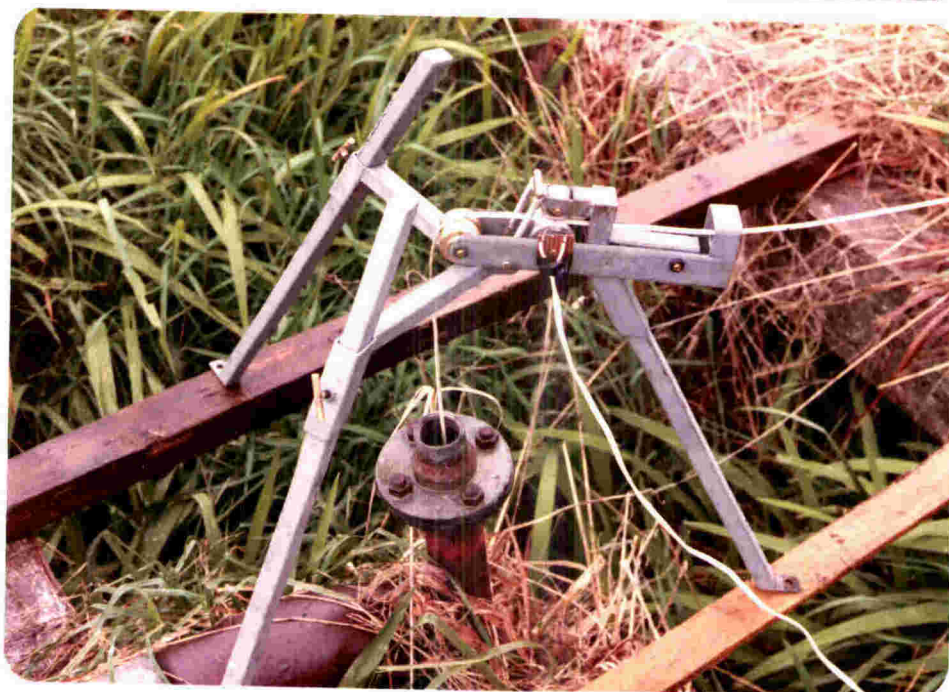
Fig. 3.1 Photographs showing borehole temperature measurement by thermistor probe.
