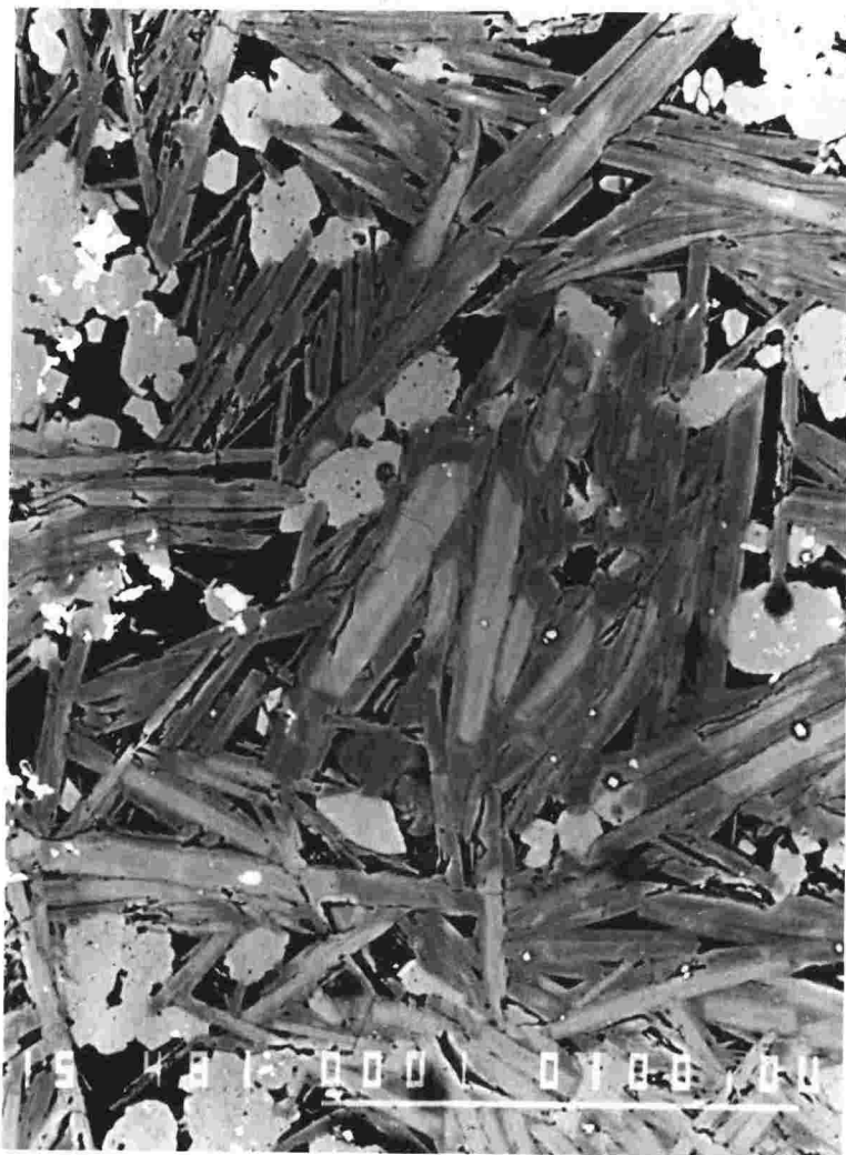
FRONTISPIECE: BEI photograph of TYPE IX xenolith (hydrothermal nodule) from Whakapapa Formation flow, Ruapehu. Minerals are natroalunite (blades), quartz (rounded aggregates) and rutile (white patches on quartz, LHS). Natroalunite is zoned with K-rich cores (lighter) and Na-rich rims (darker) Scale bar = .1mm; field of view = 1.9mm.
