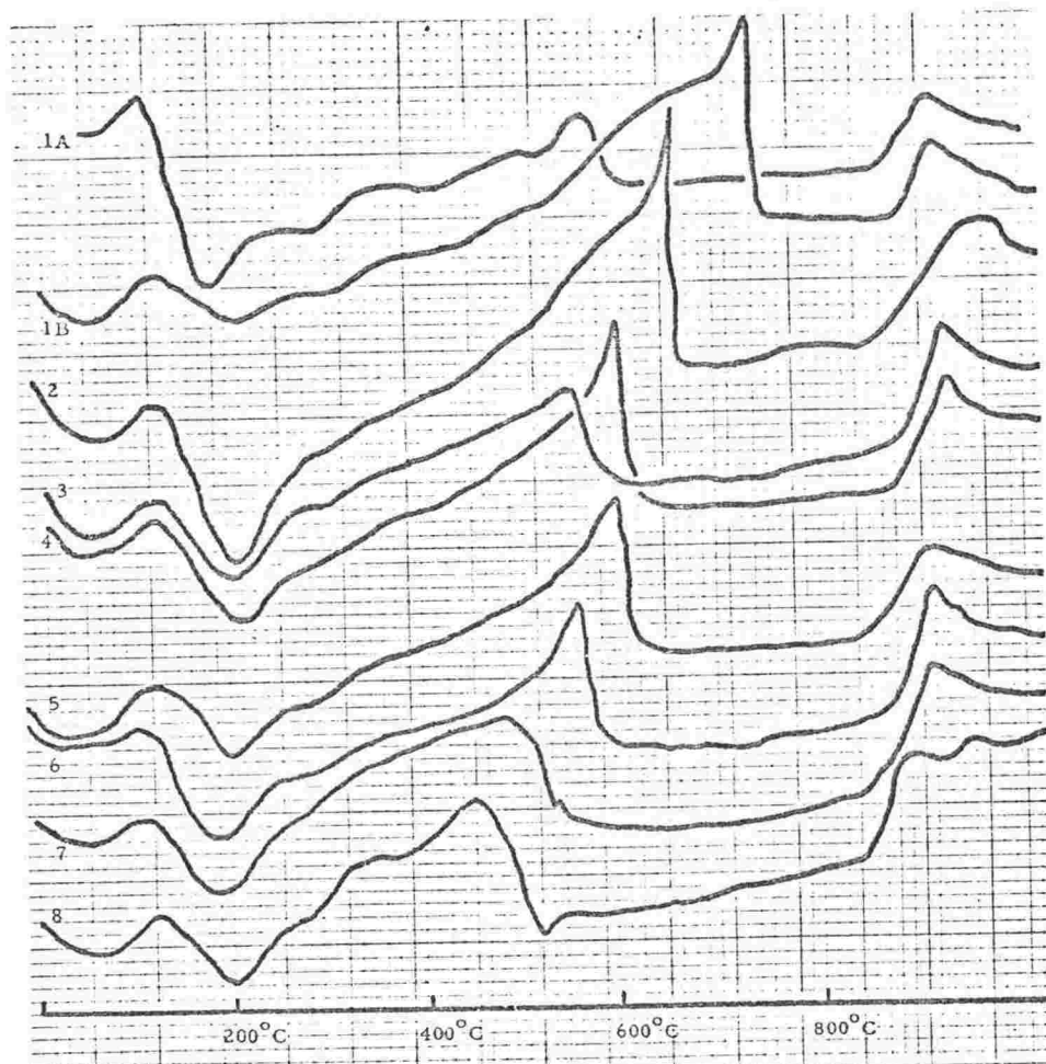
FIGURE 53 - DTA traces of clay fractions separated from selected Taranaki tephras. Traces are arranged in stratigraphic order, youngest at the top. Only the uppermost sample was treated with H_2O_2 . Sample localities refer to sections and a best locality in Neall (1972). Traces 1A ( H_2O_2 treated) and 1B (non- H_2O_2 treated) samples of Okato Tephra from Section 1; trace 2 - Koru lapilli from section 6; trace 3 - Weld ash from section 6; trace 4 - Weld ash from section 1; trace 5 - Weld tuff from its best locality; trace 6 - unnamed ash from section 6; trace 7 - unnamed ash from best locality of Weld tuff; trace 8 - uppermost New Plymouth Ash (upper part) from section 1.
