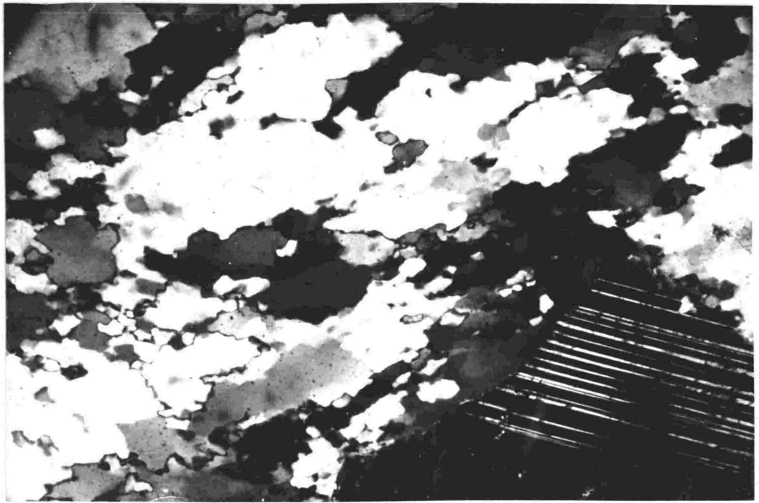
Fig. 25. Leucocratic vein showing plagioclase porphyroclasts in a matrix of quartz. Note directional fabric and undulatory extinction of quartz.
