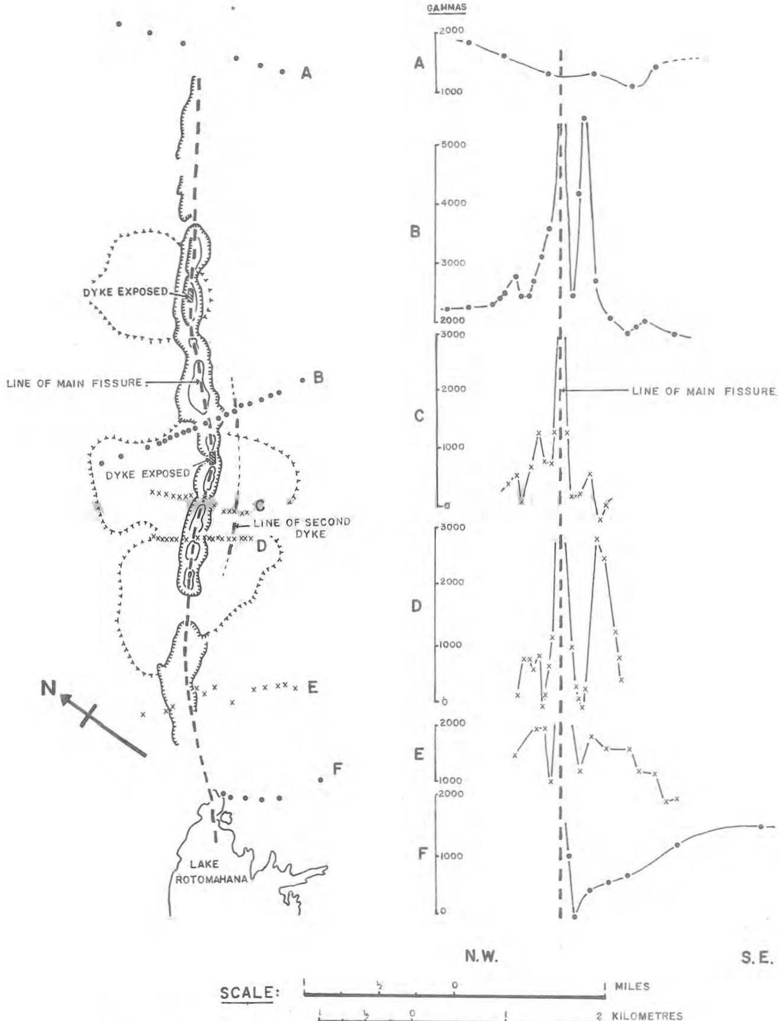
N.B. The vertical scales (in gammas) of profiles A, B and F, and those of profiles C, D and E use different zero levels and hence the two sets of anomalies cannot be directly compared.
