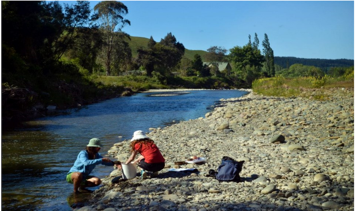
Figure 4.2: Sand collection from the Wai-iti River, a tributary to the Waimea. Samples are roughly sieved at the site to avoid collection of large sediment and a hand lens is used to estimate the amount of quartz in the sand that is collection. (Photo courtesy of Richard Jones).
