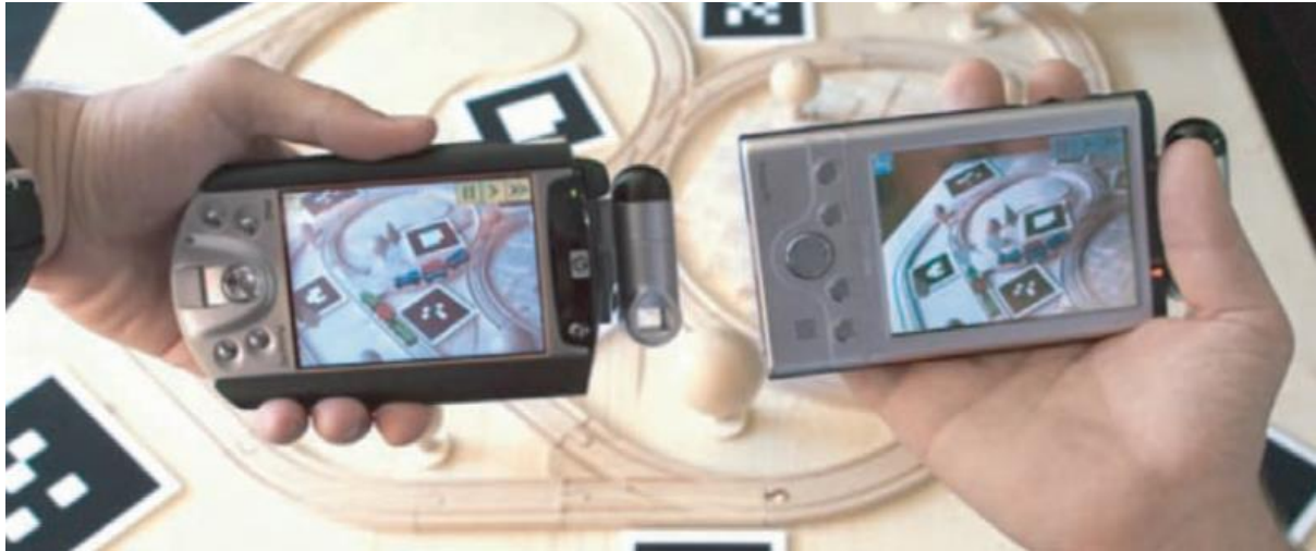
Figure 6: Early augmented reality tests: Invisible Train demonstrates collaborative hand-held augmented reality gaming (Wagner, Pinatric, Ledermann, & Schmalstieg, 2005, p. 108)
