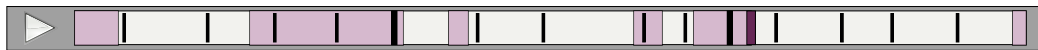
Figure 4.8: Audio Control. Thin black lines indicate segment boundaries. Thick black lines indicate row boundaries. Light purple regions indicate portions listened to. A thick purple line indicates the current play position.
