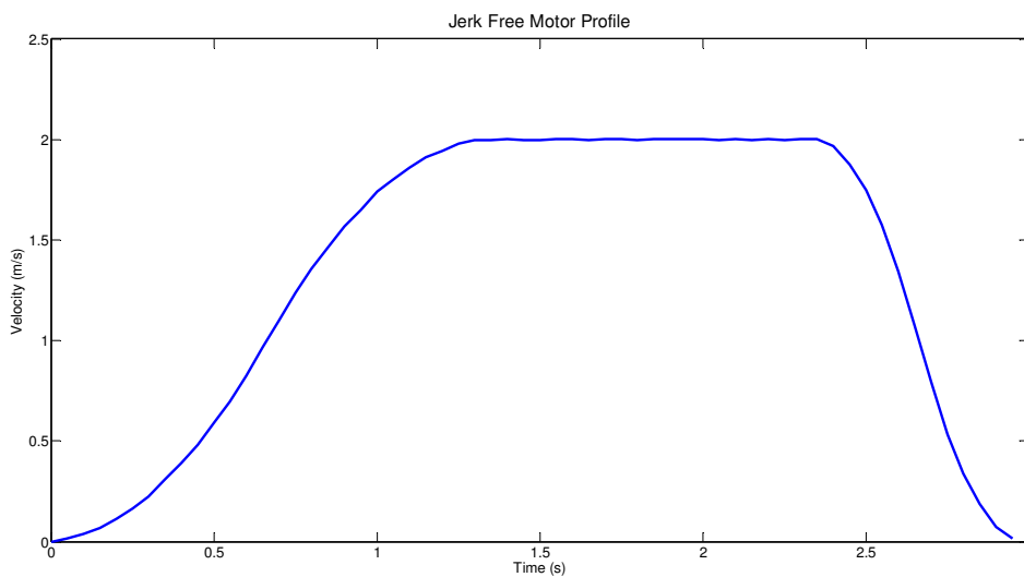
Figure 3.26 Velocity vs. Time for the fastest stable motor profile (recorded using the encoder)
