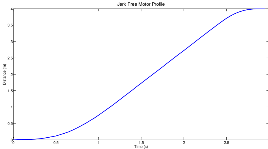
Figure 3.25 Distance vs. Time for the fastest stable motor profile (recorded using the encoder)
