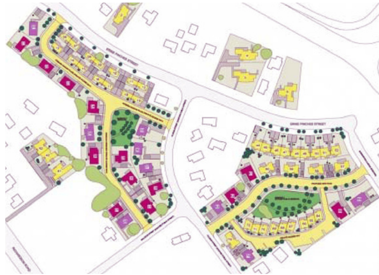
Figure 72. Master plan of Ernie Pinches Street redevelopment. Cleverly integrated with its existing suburban context, the scheme increases dwelling density, as well as connectivity and public open space (Stephenson & Turner, 2011a).
