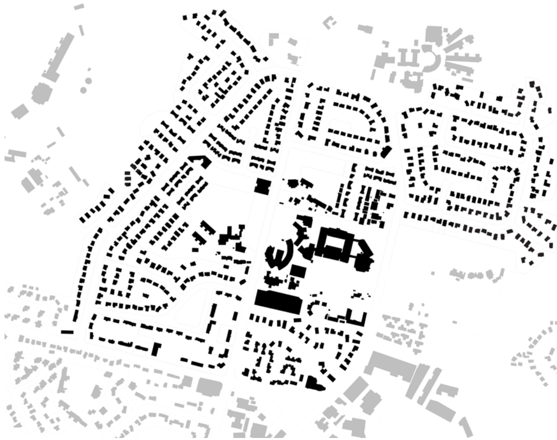
Figure 100. Post-intervention building footprint diagram illustrating how dwelling density has been increased in the design case study area through a variety of dwelling models. Note also the openness of the central community area and its connection with other open spaces and uses in the area.
