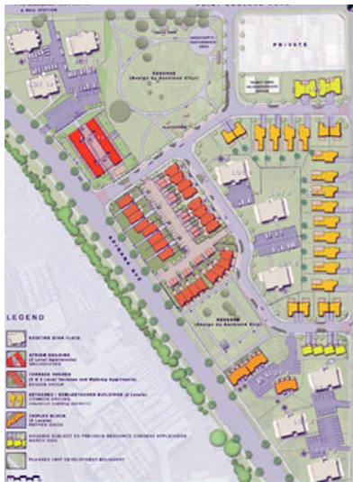
Figure 66. Master plan of Talbot Park. Note the variety of dwelling types, site permeability, and integration of public parks bordered by housing, but open to the street (Sills, 2011). Figure 67. Semi-private streetscape bound by terrace housing, with apartments and a park in the distance. Author's own image.
