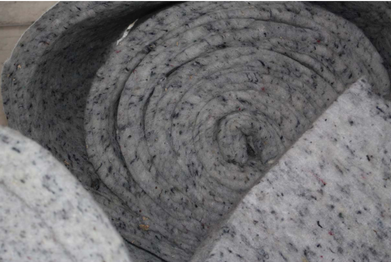
Figure 18: Ecowool insulation arrives at the construction site in Lyal Bay
