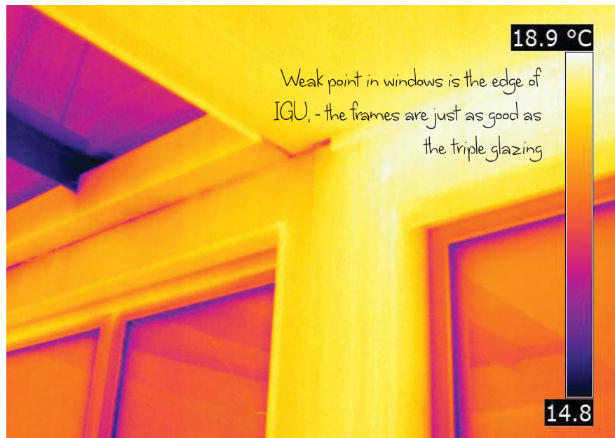
Figure 45: Thermal image of bifold doors, North facing glazing and skylight of the First Light house (Source: Image courtesy of BRANZ)
