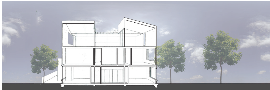
Figure 3.86 - Cross section through one house (ground floor: flexible room, laundry, bedroom, first floor: bedrooms and bathroom, second floor: living room, courtyard, dining room) Source: Authors own image
