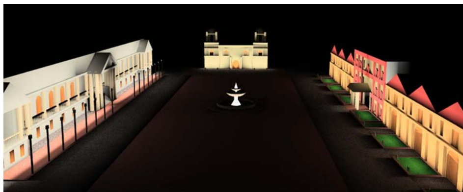
Figure 5.10 The lighting levels provided by the light coming from the façades allow the incorporation of lighting for central objects without light obstructions.
