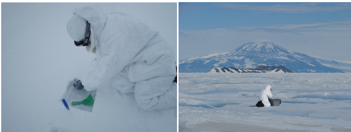
Fig. 2.17: Snow sampling procedure for bag samples, sampling downwind from Black Island and Minna Bluff, Southern McMurdo Sound, November 2009.
