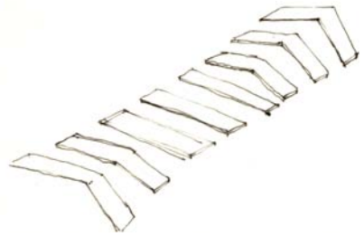
Figure 141. Directional paving provides clear visual cues to the evacuation route.
