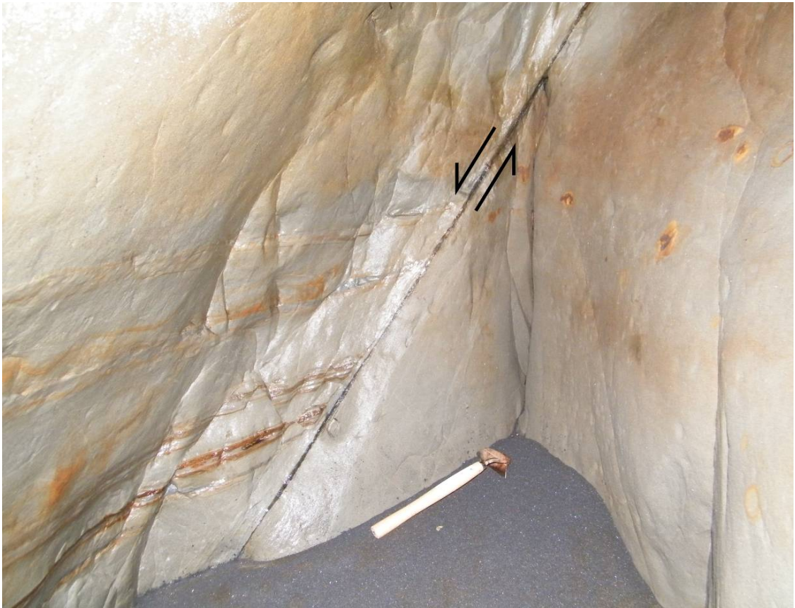
Figure 5.15 Fault Zone 3, Tongaporutu River. The fault has a single well defined slip-surface. Dark grey material defining the fault surface is fault-rock and comprises both silt and sand (some of which appears to have been smeared along the fault). Wooden tool handle is ~ 25 cm long. Location of outcrop is shown on Figure 5.3.
