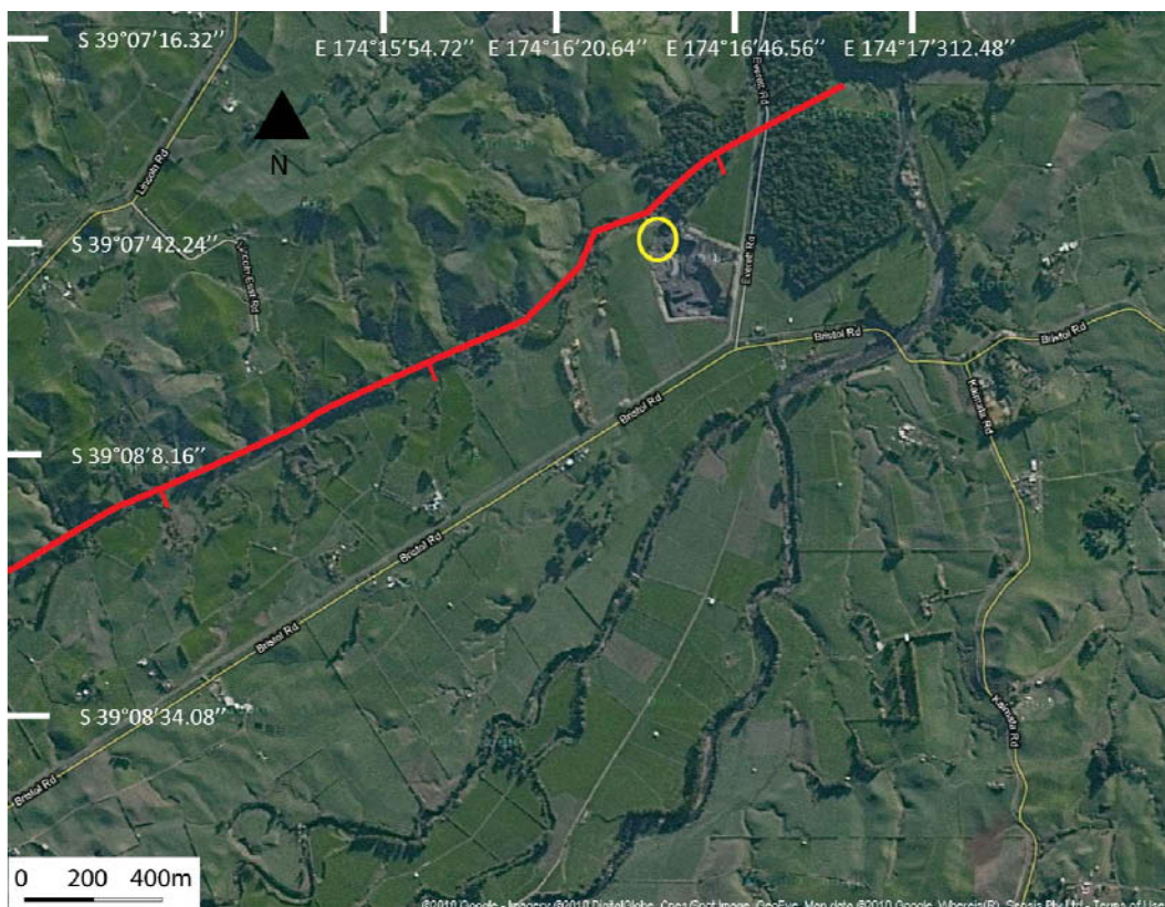
Figure 5.26 Inglewood Fault (ticks indicate down-throw and dip direction). Yellow circle highlights the location of oil and gas surface leak in Bristol Road Quarry. Image adapted from Google Maps ( www.maps.google.com ). Location of image is shown in Figure 5.2.
