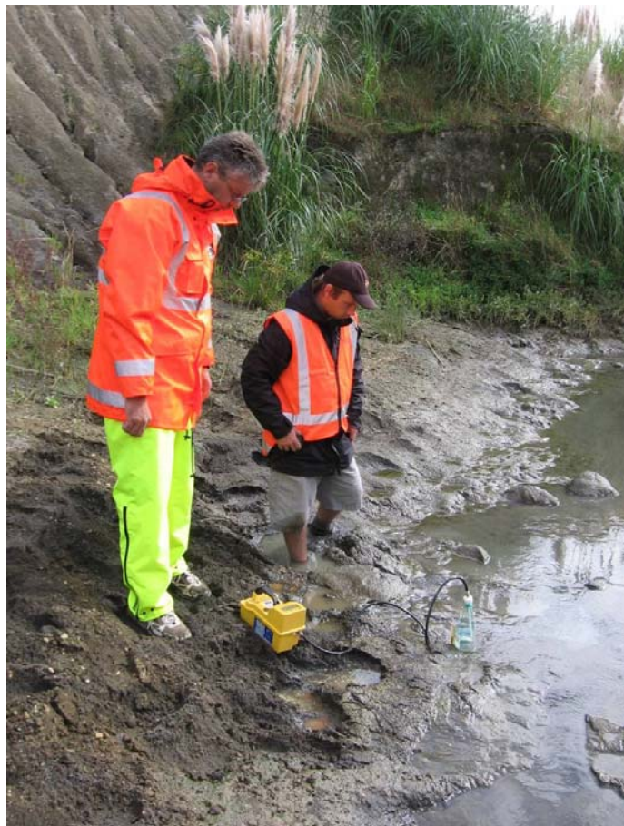
Figure 5.29 Operating the gas sniffer in the floor of the Bristol Road Quarry.
