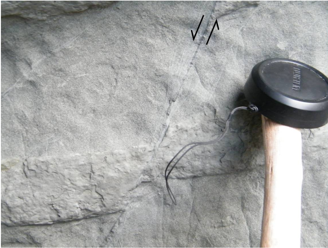
Figure 5.14 Minor fault in the foot-wall of Fault Zone 2. Deformation bands in the sandstone enclose the primary slip-surface which towards the top of the photo is defined by dark grey fault-rock. Arrows indicate slip sense along the fault. Lens cap is ~ 6 cm diameter.
