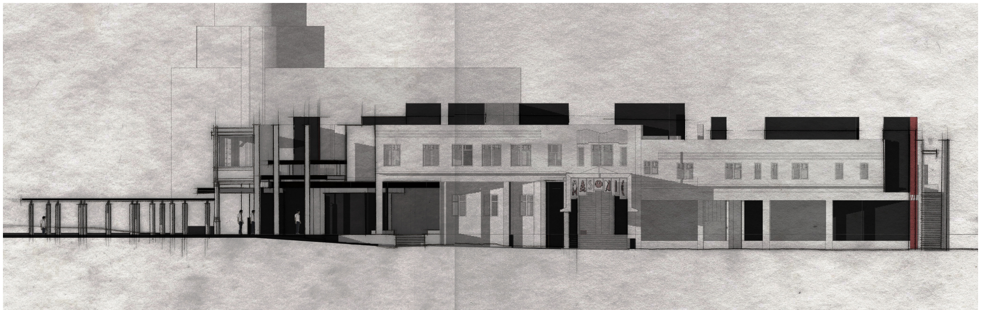
Figure 74. Tennyson Street Elevation. The Dark elements highlight the changes that have been made to the original building. Image by Author, 2010.
