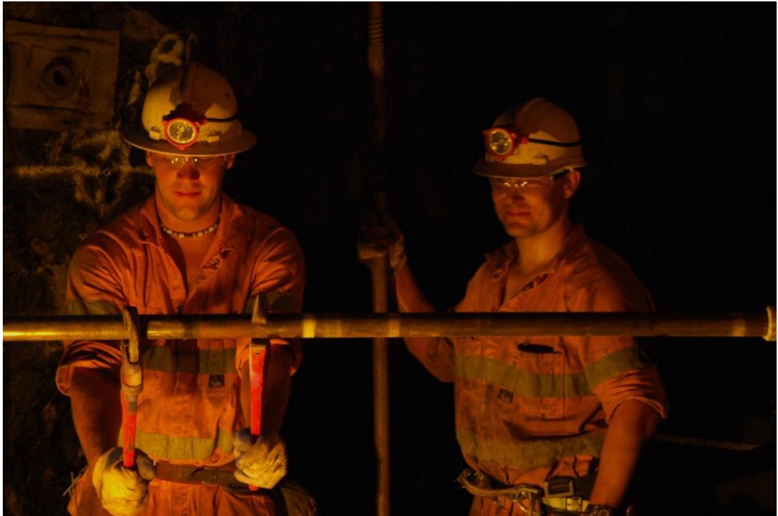
Diamond drillers cracking a drill string.
