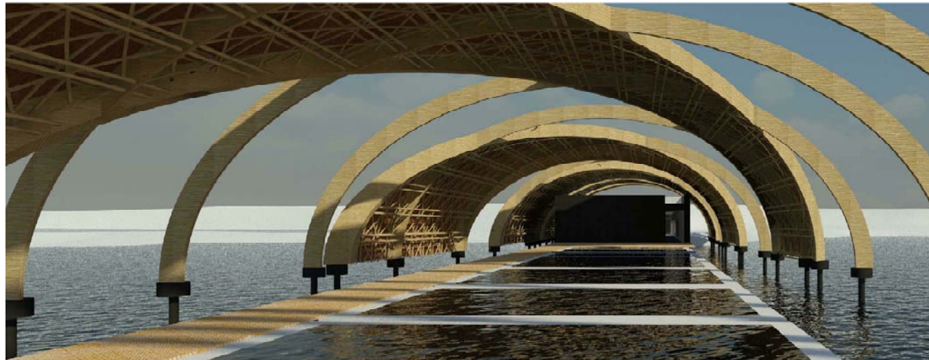
Top Refined design showing integration between natural bamboo, laminated bamboo and BMB
