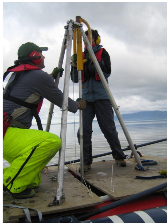
Fig. 8 - Corer being manually driven into the lakebed from the flat wooden deck of the cataraft (Photo: Marcus Vandergoes, GNS).
