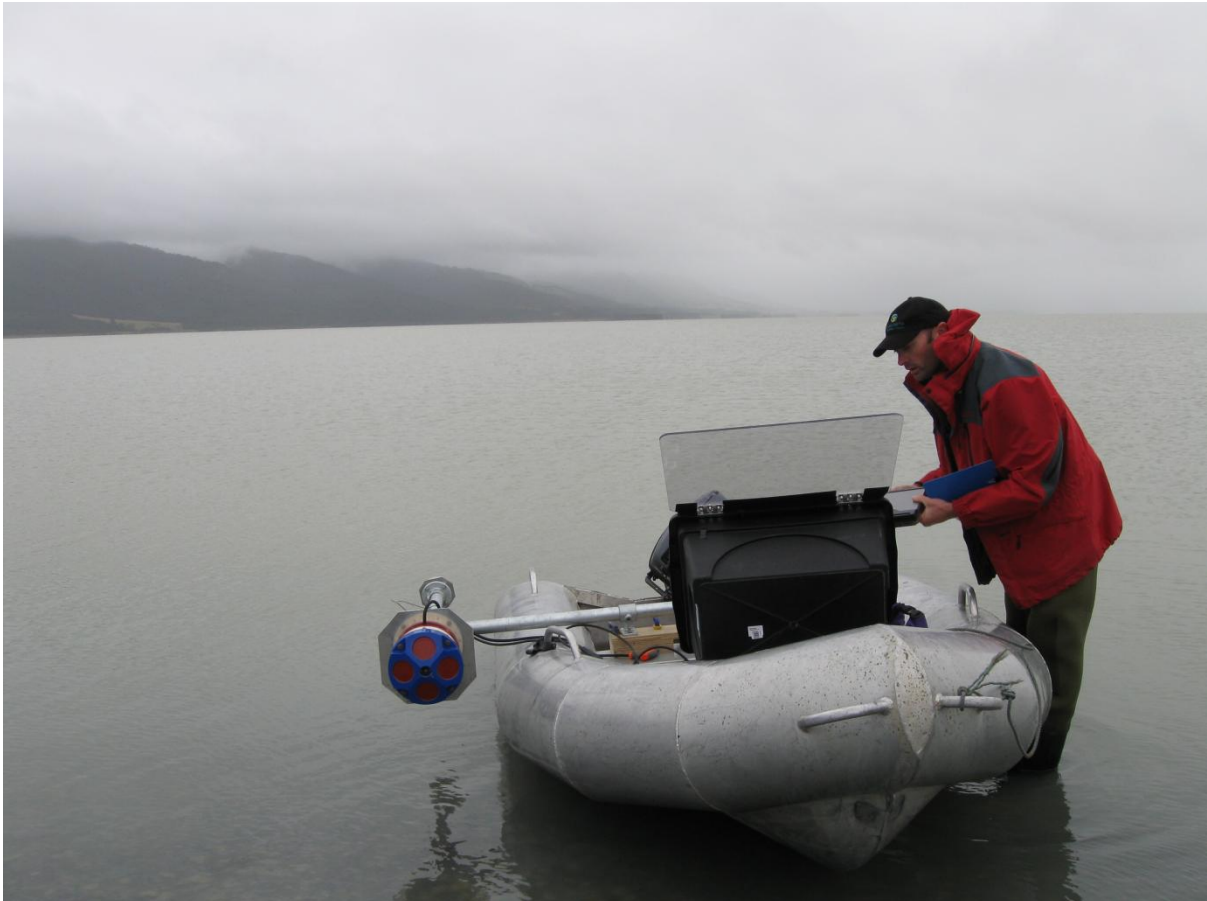
Fig. 6 - Acoustic doppler current meter (ADCM) attached to the boat. Once the boat is pushed into deeper water the ADCM is positioned vertically so that the blue and red sensor sits at the water surface. The computer is positioned in the black box at the front of the boat (Photo: Des Peterson, GWRC).
