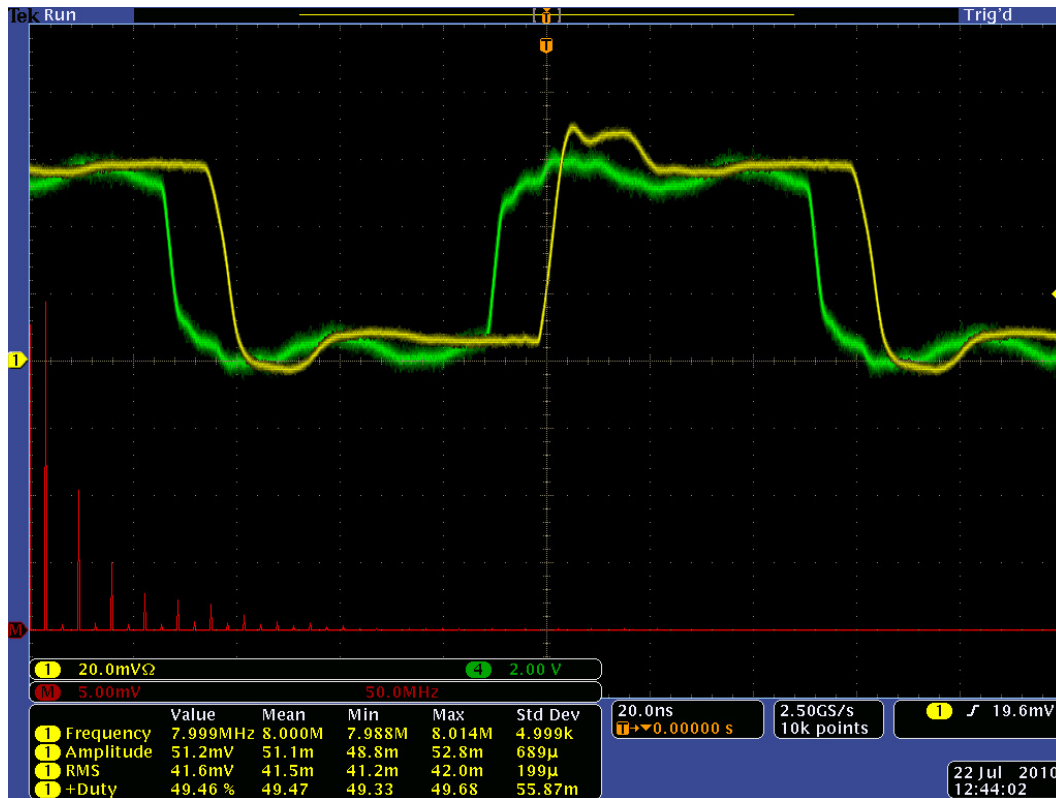
Figure 4.1: Laser diode illumination waveform with modulation frequency of 8 MHz as measured by a photodiode.
