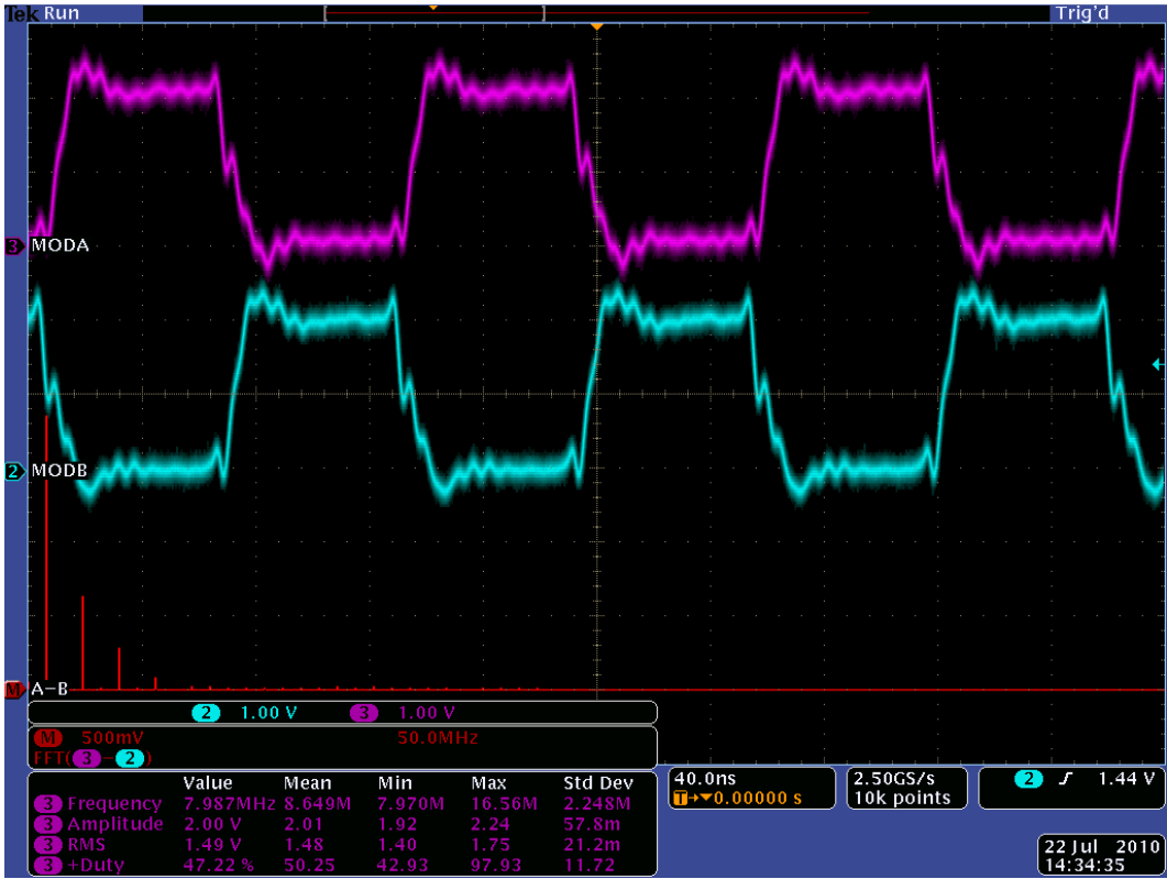
Figure 4.3: PMD19k sensor modulation waveform with frequency of 8 MHz. Purple and blue traces show the voltage of the A and B modulation inputs respectively. Red trace shows the FFT of their difference.
