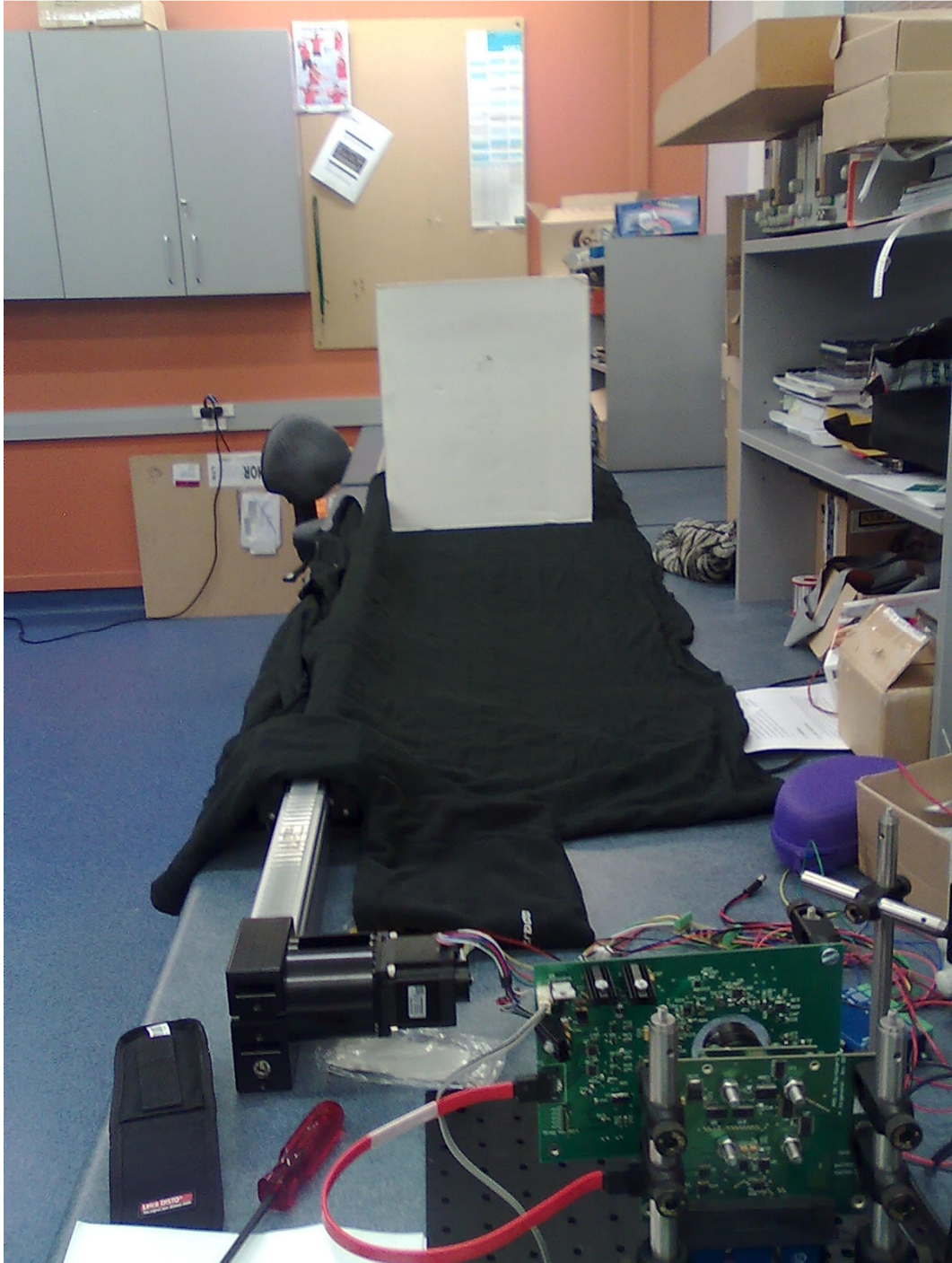
Figure 4.7: Simple static test scene used for characterising tests. In the centre of the field of view is a single white rectangular target, positioned 2.63 m from the range imaging system.
