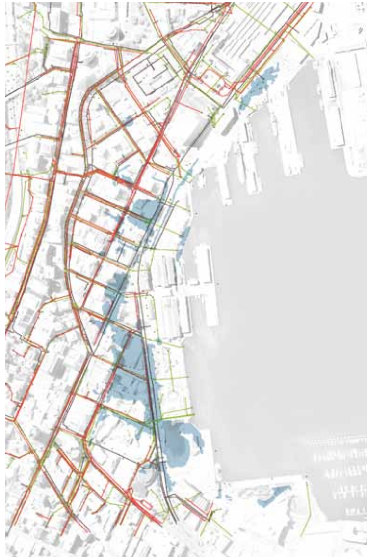
Fig 6.12 Infrastructure — Drainage - sewer pipes + nodes — Drainage - stormwater pipes + nodes — Water network pipes + nodes
