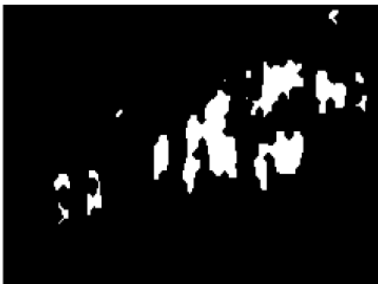
Figure 6.3: After the background subtraction step, from the image in Figure 6.2 a binary image of the foreground is used to extract observations for the tracking algorithm. A single blob might contain either a group or a single person.
