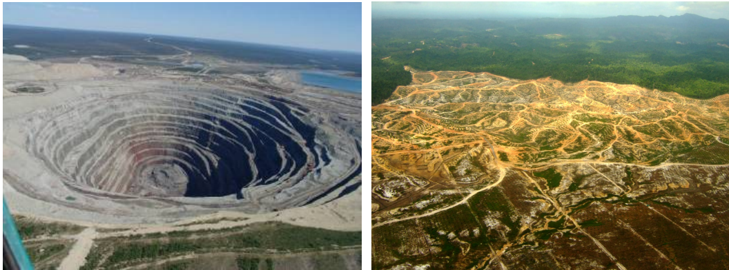
Figure 1: Open pit diamond mine located in Mirny, Eastern Siberia and rainforest destruction in Borneo. The mine is 525 m deep and has a diameter of 1200 m.
