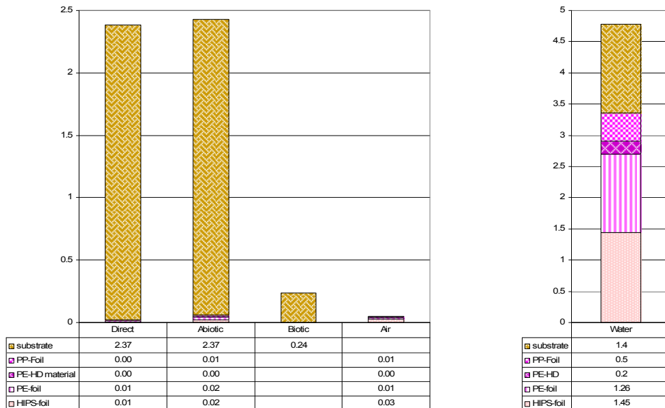
Figure 91: Resource use of the green roof of the multifunctional envelope (excluding roof structure) over 60 years (in tonnes)
