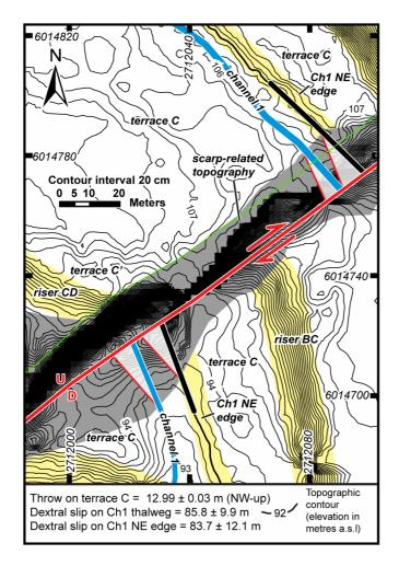
Figure 11d. Microtopographic map of terrace C and Ch1 displacements across the Wairarapa Fault. See Figure 3 for location. Map is based on a survey data set consisting of ~3620 points, which are omitted for clarity. On this topographic map the contour interval is 20 cm.
