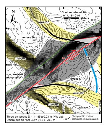
Figure 11c. Microtopographic map of and riser CD terrace displacements across the Wairarapa Fault. See Figure 3 for location. Map is based on a survey data set consisting of ~2920 points, which are omitted for clarity. On this topographic map the contour interval is 20 cm.
