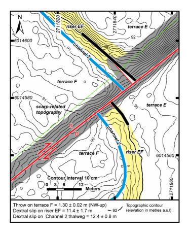
Figure 11a. Microtopographic map of terrace F, riser EF and Ch2 displacements across the Wairarapa Fault. See Figure 3 for location. Map is based on a survey data set consisting of ~4900 points, which are omitted for clarity. On this topographic map the contour interval is 10 cm. Projection uncertainty on downthrown side is too smale for map scale. Elevations are metres above sea level (m asl). Coordinates are in NZMG.
