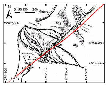
Figure 4b. Grapes and Wellman's (1988) interpretation of the terraces at Waiohine River. Seven terraces were identified (ag3 and a-f). Three distinct paleochannels incised into ag3 (Waiohine surface) were identified, displaying ~130 m dextral displacement. Depressions are indicated stippled by areas. Wairarapa Fault is in red. Terrace edge/top of fault scarp is in green. Coordinates are in NZMG.
