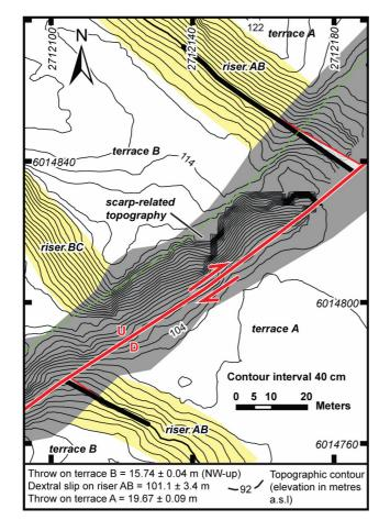
Figure 11f. Microtopographic map of terrace A, terrace B and riser AB displacements across the Wairarapa Fault. See Figure 3 for location. Map is based on a survey data set consisting of ~2790 points, which are omitted for clarity. On this topographic map the contour interval is 40 cm.
