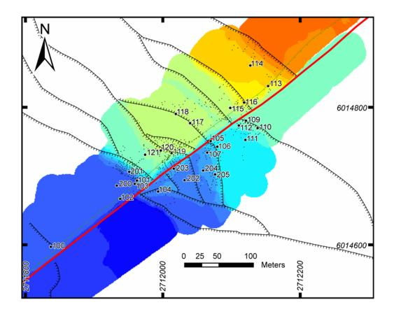
Figure A3-1. EDM control points and survey points from the 2007 (100-121) and 2008 surveys at the Waiohine terraces. Labelled large black circles are EDM control points, locations of which were determined during 2007 and 2008 RTK GPS surveys. Small black circles show entire EDM data set collected during the 2007 and 2008 surveys. Control point 108 was removed from the survey and is not shown.
