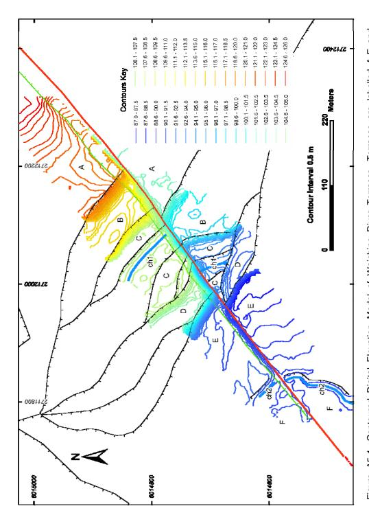
Figure A5-1. Contoured Digital Elevation Model of Waiohine River Terraces. Terraces are labelled A-F and paleochannels are labelled ch1 and ch2.
