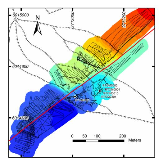
Figure A1-1. RTK base stations and survey points from the 2008 surveys at the Waiohine terraces. All base stations in these surveys were set up over the same marker peg at the Waiohine terraces, with the exception of RTCM0001. Large black circles are RTK base stations. Small black circles show entire RTK data set collected during the 2007 and 2008 surveys.
