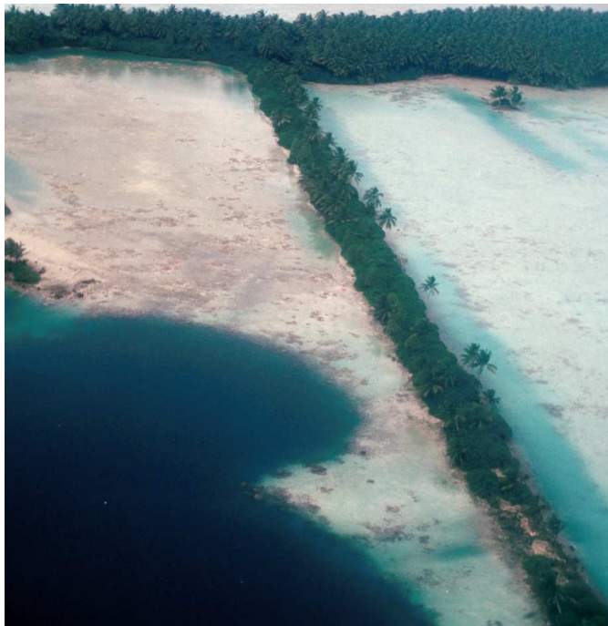
Fig 4.8 Aerial view of northern part of the North-South Causeway between Center and East lagoons looking north, taken in 1979. Patch reef material has been removed from a
