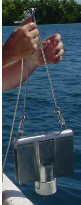
Fig 3.1 Photo of dredge used to retrieve sediment from the lagoon substrate. The 1 cm deep openings at the front collect only the surficial layer of sediment.
