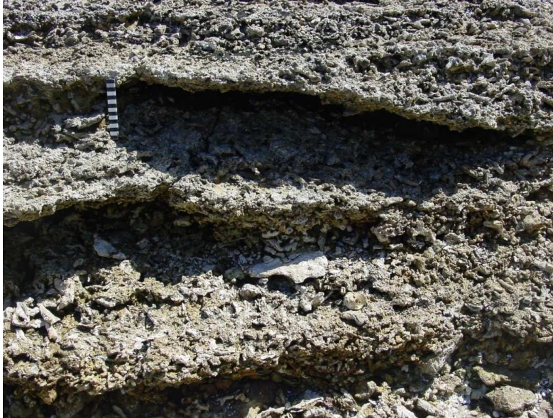
Fig 4.20 Typical beachrock showing stratification, southern coast of Paradise Island Indicator denotes 10 cm.
